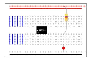
The above diagram shows how the holes of a breadboard are connected. The bottom and the top rows are connected horizontally across as the red and the black line denotes. The power supply is connected to both the black and red rows. The other rows are connected in a vertical manner which consists of five rows each without any links to the across the centre. In this way there are separate blocks of connections to each of the ICs pin. Now this was the connection in a small breadboard.
