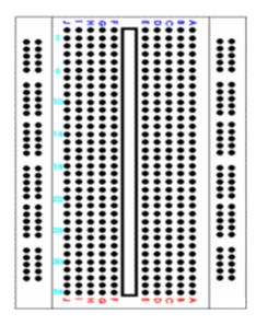
In the below diagram you can see both the vertical columns and horizontal to be connected internally. As soon as the power
